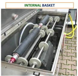
Our "ORION" model washing machine has been designed to meet the needs of companies in the LABEL PRINTING sector that need to wash cylinders, inking trays, side covers and doctor blades.
