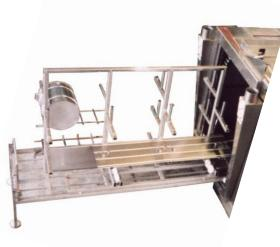
Our washing tunnel model "LIBRA" has been specifically designed for components coming from Roto and Flexo printing machines (inking trays, side covers, ink tanks, doctor blades, tools and other components).
